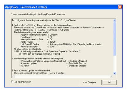
**NOTE.** The CPU is used 100 % when the MPEG Player plays in IP mode with TS bit rate more than 10 Mbps. During this playout, duplex operation is not possible, so TSCA cannot be run.
