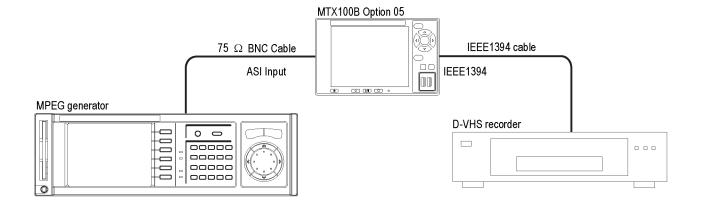
Figure 33: Connection example for ASI to IEEE1394 conversion
