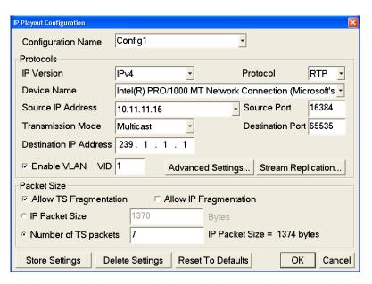
Figure 8: IP Configuration for IPv4
