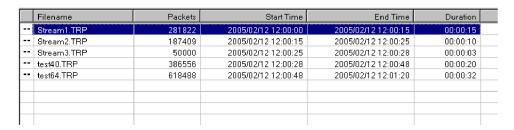
If you set a Start Time (for example, 2005/2/10 15:00:00) in the Play Properties dialog box for an individual stream, the start date/time of all subsequent streams are changed. This does not affect the preceding streams.
