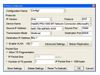
Figure 9: IP Configuration for IPv6
