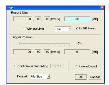
**Target Dialog Box.** When you select the Target command from the Record menu, the Target dialog box appears. (See Figure 21.)
