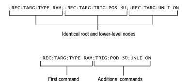
Figure 28: Example of omitting root and lower-level nodes in a chained message
