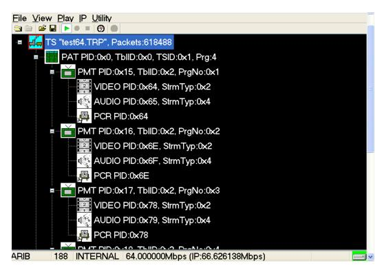
The "+" symbol displayed to the left of some icons indicates that the item includes lower-level transport stream components that are not displayed. The symbol changes to "—" when the lower level components are displayed. To expand the hierarchy, select the desired upper-level icon and press the right control button. To collapse the selected upper-level icon press the left control button.
