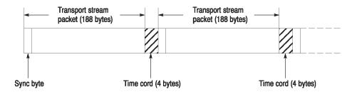
Figure 35: Partial transport stream
