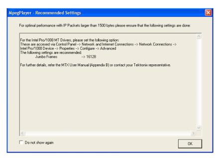
■ **IP Packet Size**: Allows you to set the size of the IP packet for playout. This option is enabled only when Allow TS fragmentation is selected. The maximum size of the IP packet for IPv6 version is 16128 bytes and for IPv4 version is 1500 bytes.
