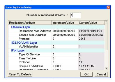
Figure 12: Stream Replication Settings for IPv4
