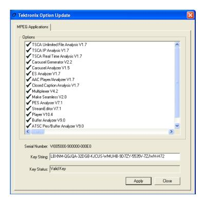
The MTX100B MPEG player and recorder is shipped from the factory with the appropriate Option Key already applied to support all of the functions that were ordered. The Option Key is documented on the Tektronix Authorization Key Certificate that is shipped with the instrument and on the top cover label of the instrument.
