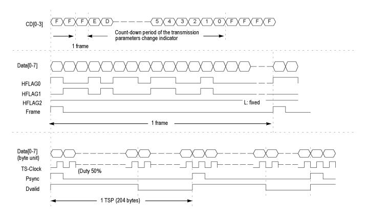
Figure 67: Timing relationship of the signals on the Universal In/Out connector
